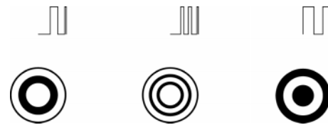
Figure 2. Example Registration Marks and Corresponding Radial Profiles
